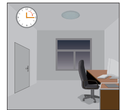
Light switches off automatically after the Stand-by dimming time elapses (unless dimming time is set to infinity).
