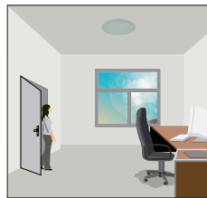
With sufficient natural light, the light does not switch on when a presence is detected.
