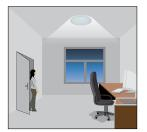
With insufficient natural light, the sensor switches on the light automatically when a presence is detected.
