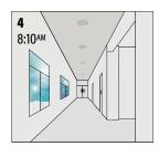
When the natural light level exceeds set point off to light,the light will turn off even if when the space is occupied.
