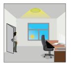
When natural light is sufficient or dark, and movement is detected the light will turn on to 100% brightness.
