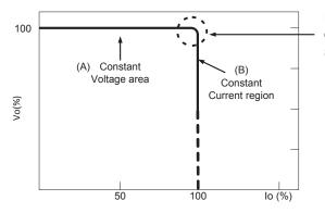
Typical LED power supply I-V curve
