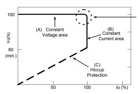
Typical LED power supply I-V curve
