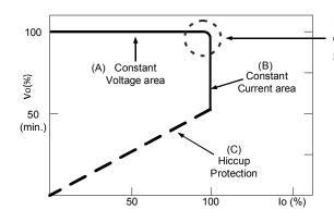
Typical LED power supply I-V curve
