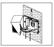
5. Replace the lens set on the hinge and finish connection, Close the lens set and tighten the screws to fasten the lens set to the back plate.
