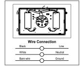
4. Finish wiring (Black for Line, White for Neutral and Bare wire for Ground).
