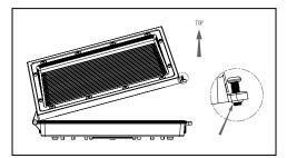
1. Loosen screws and remove the front lens set carefully from the back plate.
