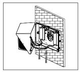
5. Replace the lens on the hinges, make connections and close the lens set then tighten the screws.
