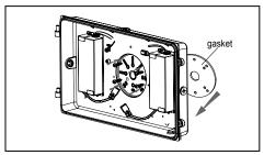
2. Drill appropriate knockouts (B) for wiring, the fixture supports standard 3 1/4" and 4"Junction box.
