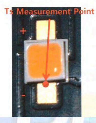
LED Lighting Source In Situ Temperature Measurement
