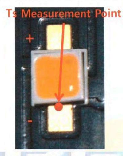
LED Lighting Source In Situ Temperature Measurement
