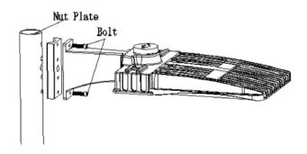
1. Drill holes on the round pole corresponding to the holes on the arm, and use the bolt and nut plate to fix the fixture to the pole tightly.
