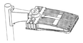
2. Connect the AC wire of the fixture and tighten the water-proof gasket and cover plate on the arm by screws, then power on.
