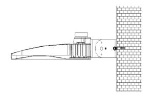
2. After securing bracket to the wall angle can be adjusted by the small screw on the side (make sure to tighten screws after desired angle has been set), then connect the AC wire.
