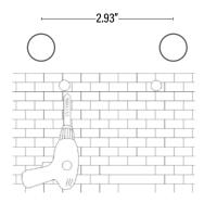
**1.** Drill 2 holes in the wall to match the mounting holes on the trunnion bracket. Use expansion screws/anchors to properly secure it to the wall.
