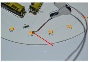
Temperature measurement point of LED board (TMP<sub>b</sub>)
