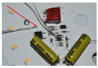
Temperature measurement point of driver (TMP<sub>c</sub>)
