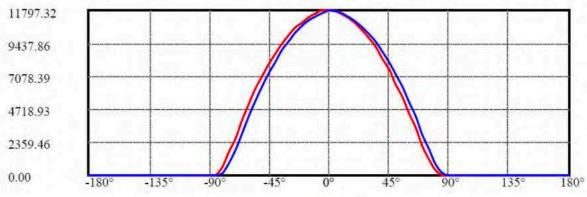
Field angle(10%Imax):C0/180Left:77.1 Right:74.6 :C90/270Left:73.2 Right:78.3 Beam Angle(50%Imax):C0/180Left:56.2 Right:53.3 :C90/270Left:52.1 Right:57.0
