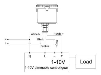
\*The sensor is designed for connect one load only. Connect more than one loads may damage the sensor.
