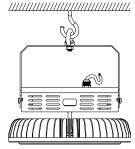
2. Secure hook to the ceiling and hang the fixture from the hook.
