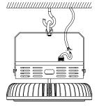
3. Connect the electrical cables; Black-L, White-N, Green-Ground. If using in wet locations, ensure all electrical connections and installation holes have a water tight seal.
