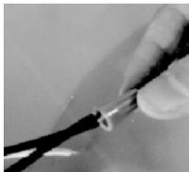
STEP 3: Insert male connector into female one.
