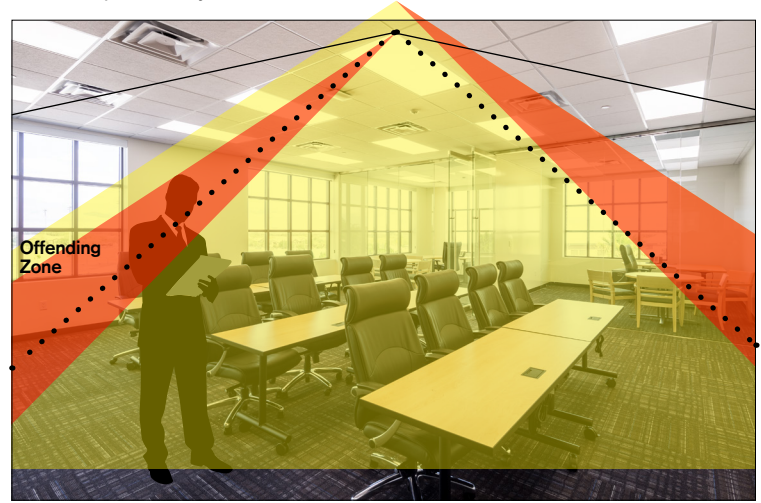
■ = High glare flat panel makes occupant's eyes feel uncomfortable — = 90° ..... = 60°
