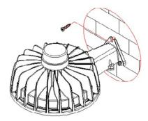
3. Hook the lamp by two screws, fix the top screw, finally tighten all screw
