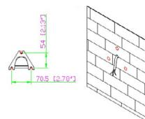
1. First refer to the size of the diagram to bore a hole on the wall
