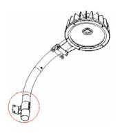
5. Fixed clamp on the pipe in a right position and make sure that the pipe will not rotate.
