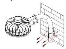
6. Install the light fixture on the wall with four screws.
