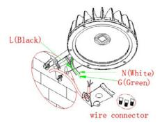
4. Pass the wire through the hole of the cover plate, connect the wire in same color (correspond to wire N, L and G) together with a wire connector.
