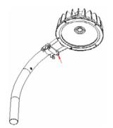
4. Put one end of the tube into the U-slot, and then fix the tube with two hex socket screws. Please make sure that the tube will not rotate.
