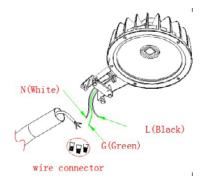
3. Connect the wire in same color (correspond to wire N, L and G) together with a wire connector.
