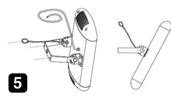
If you are installing the fixture to a wall stud or vertical post, attach fixture using 2 bolts or screws (not provided) and mounting holes on hanging bracket as shown. Chosen hardware and mounting surface must be capable of supporting 22lbs (10kgs) if hanging a 160W or 250W model. Secure safety cable to wall stud or vertical post using another set of hardware (not provided) with the same support capabilities as the installation hardware.
