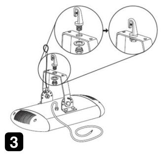
Adjust hanging bracket to desired angle. Secure angle by inserting bolt from safety cable assembly in Step 1, and additional included bolt through fixture bracket hole in hanging bracket leg as shown.
