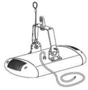
Attach the fixture hook to your structural beam or stud using hardware (not provided) that is capable of supporting 22lbs (10kgs) if hanging a 160W or 250W model Secure safety cable to structural beam or stud using another set of hardware (not provided) with the same support capabilities as the installation hardware.
