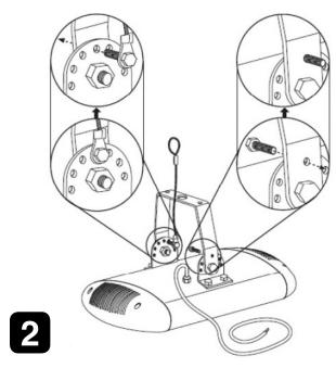
Adjust hanging bracket to desired angle. Secure angle by inserting bolt from safety cable assembly in Step 1, and additional included bolt through fixture bracket hole in hanging bracket leg as shown.
