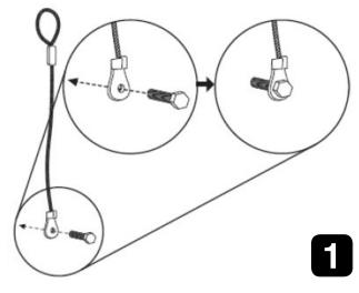
Slide end of safety cable over one of the included bolts as shown
