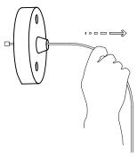
8. Put the upper suspended rope into the hole of the flange to insure the end cap inside the flange.
