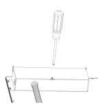
5. Fix the cover of the Junction Box then tighten the screw
