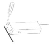
1. Remove the screw on both ends of the Junction Box, then make the right hole for wire.
