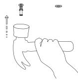
7. Put the expanded screw into the hole, insure the external rim is aligned with the wall.
