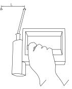
6. According to the specification, slotting a hole on the ceiling as the photo shows, diameter 0.24" in (6mm) by 1.38" in (35mm) deep.
