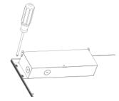
1. Remove the screw on both ends of the Junction Box, then make the right hole for wire.
