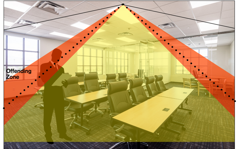
■ = High glare flat panel makes occupant's eyes feel uncomfortable — = 90° ..... = 60°
